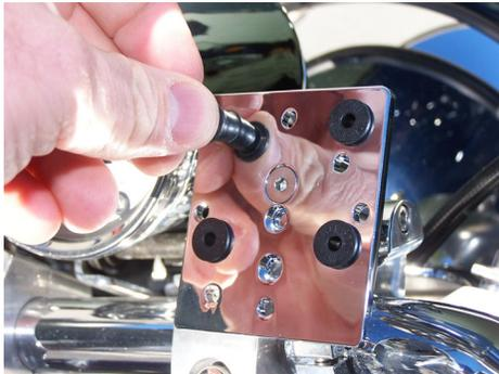
If you're using the TechMount to hold a Garmin StreetPilot GPS or a Delphi XM Radio, you may find that the device you want to mount has four holes in the back that line up with the four large holes on the TechMount plate.
