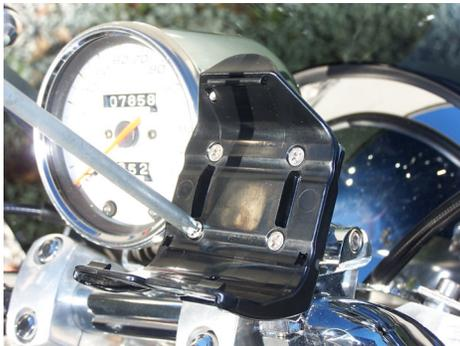
Put the four expansion nuts in from the front, as shown. Then put the device you want to install on top of the nuts, and run the screws through the device and into the expansion nuts. As you tighten the screws, the expansion nut will bulge, holding the whole assembly together. Do not overtighten; you will want a little "give" in the expansion nuts to absorb vibration while riding.
